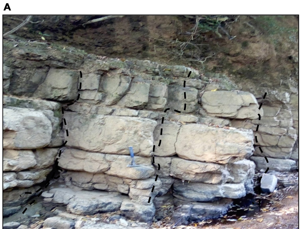
Fig. 6 A Photograph showing mine face exposure of limestone at an excavation site at 135 communities about 800 m from the 135 junction, Umuebe. The black dashes shows the fracture trend observed on the rock. B Showing rock exposure at the excavation site in Anya mmaya village Ezzamgbo
