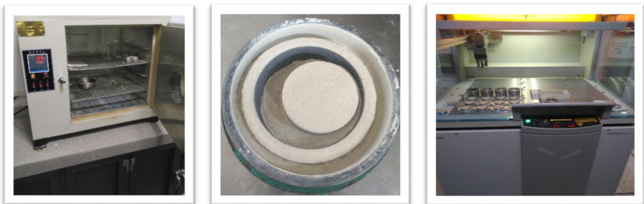
Fig. 5 Left—drying of the samples in the oven, middle—a crushed sample, right—XRF equipment
