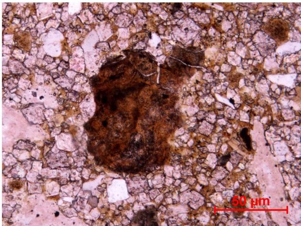
Fig. 8 Assemblage of calcite, dolomite (iron-stained rhombohedral crystals), opaques, and quartz (colourless) associating collophane. Collophane (brown grains, pellets, spheroids, ovoids) is growing at the expense of carbonates. Notice that the boundaries of collophane are convex towards carbonates. PPL
