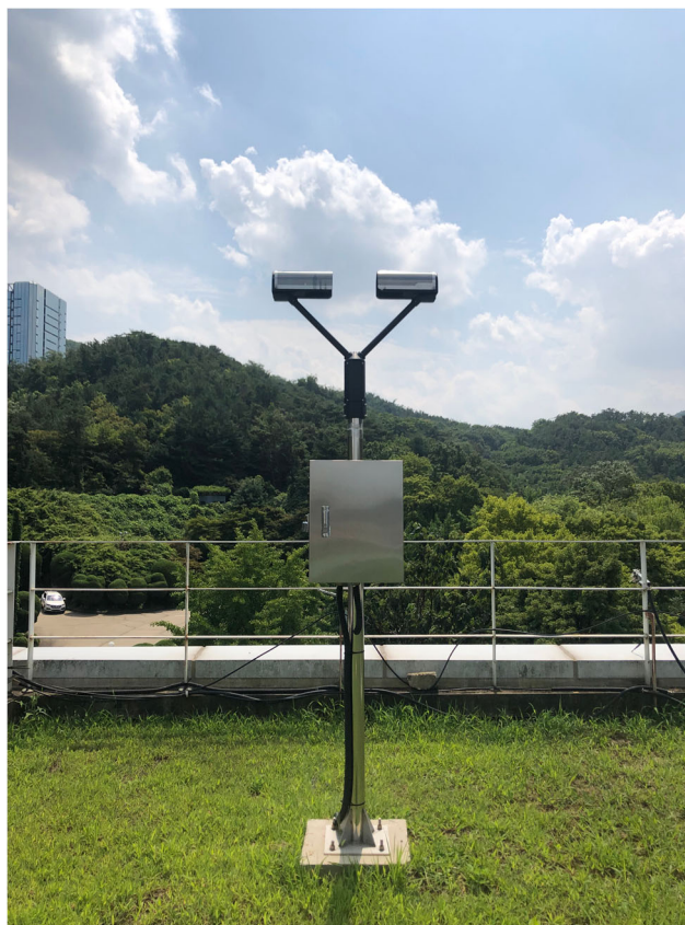
Fig. 1 Photo of the disdrometer installed on the roof of the Atmospheric Environmental Observatory building, Seoul National University
