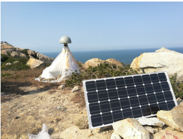
Fig. 2. GPS reference station installed in Zhiwan Island, and a solar cell for power supply.
