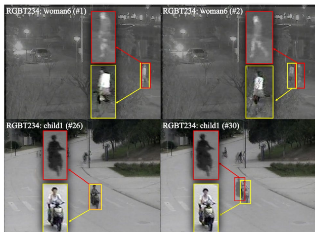
Fig. 1 Superimposed image of infrared and visible light image pair. The weight of the visible light image is 0.6, and the weight of the infrared image is 0.4. The object in the yellow box with rich texture, details, and color is from the visible light image. The object in the red box, which the silhouette can roughly distinguish, is from the infrared image
