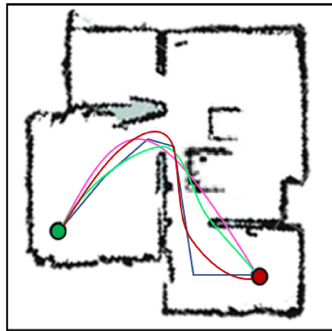
(t) Path smoothing with conventional method CBG, PMBC and proposed SPT (Red)
