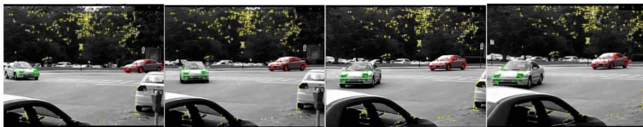
Fig. 1 Several Image Frames from Cars5 Sequence in the Hopkins155 Motion Dataset. Different color segmentation feature points represent different moving objects (colour figure online)
