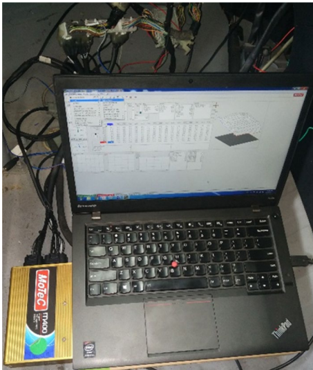
Fig. 13 MoTeC M400 ECU for engine basic control
