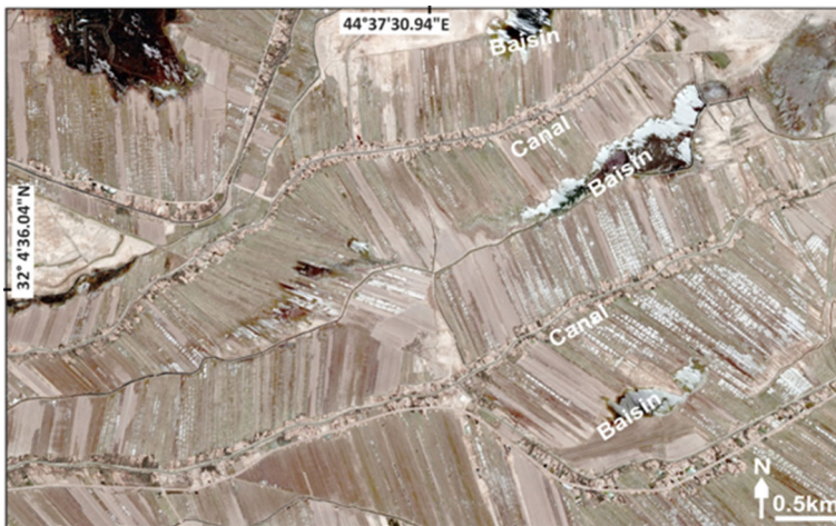
Fig. 4 Herringbone pattern of fields in the western plains showing the canals on raised ground and the basin soils between. Note occasional areas of salinization around some basin areas (by Jaafar Jotheri)
