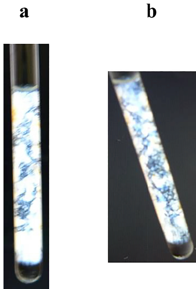
Fig. 2 The polarized microscopy pictures for two lyotropic systems based on \text{C}_8\text{E}_5 (a) and \text{C}_{12}\text{E}_5 (b)
