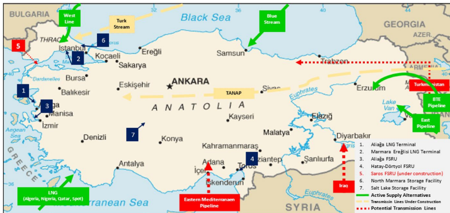
Fig. 16 Natural gas supply network of Turkey
