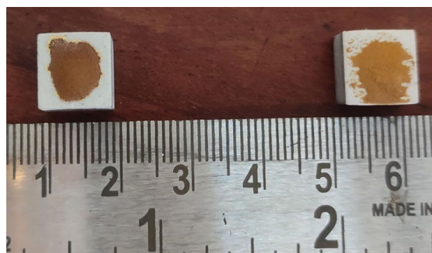
Fig. 1 The TBC samples with corrosive salts applied over the surface
