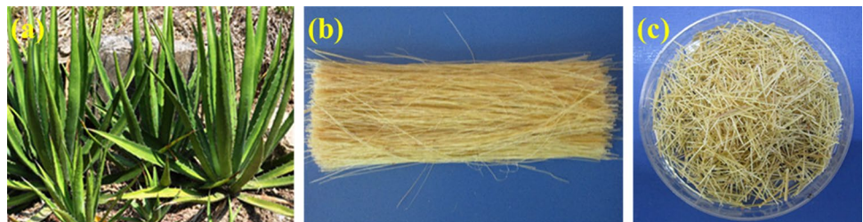
Fig. 2 a Agave lechuguilla plant b Agave lechuguilla long fiber c Agave lechuguilla short fiber
