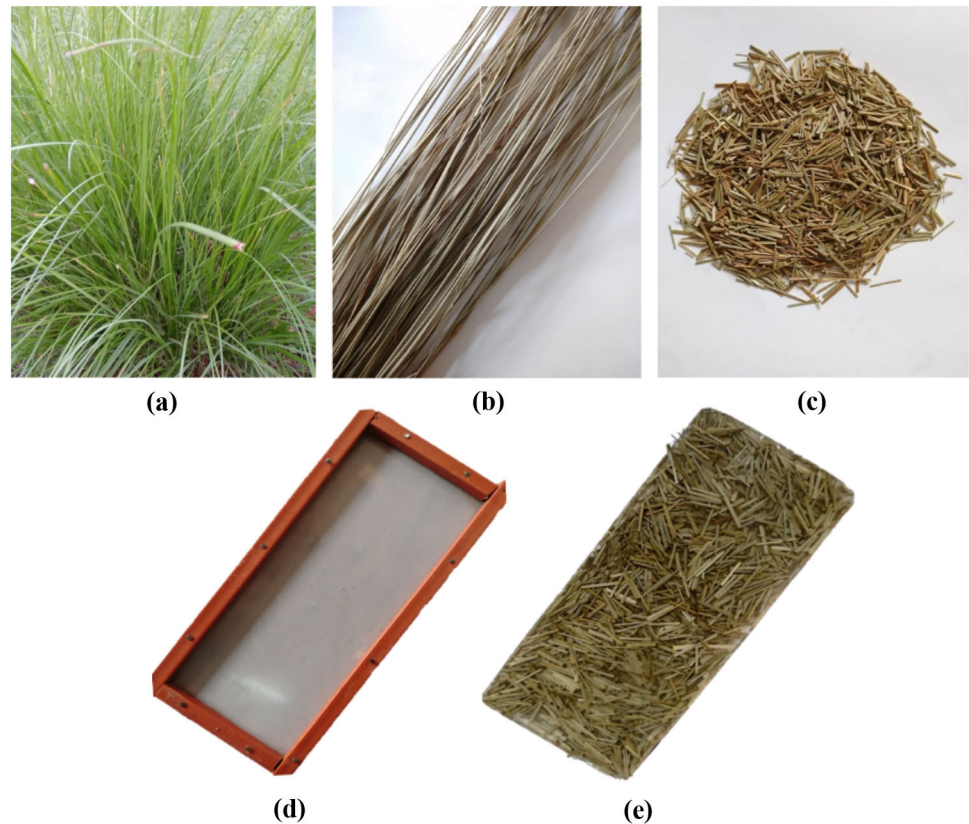
Fig. 1 a Eulaliopsis Binata plant, b long fiber stems, c short EB fiber, d wooden mold and e fabricated EB fiber epoxy composite slab
