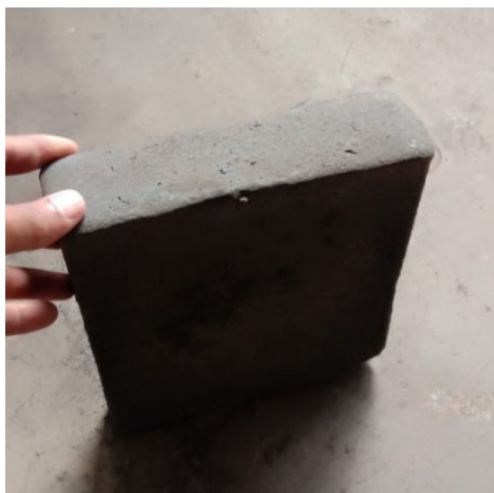
Fig. 1 As-cast Y-block after shakeout from mould
