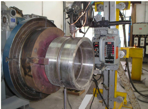
Fig. 2 Photograph image of the torch manipulator and pipe holding fixture
