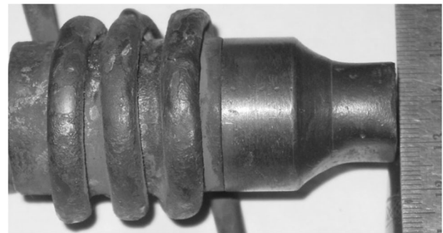
Fig. 3 Photograph showing GMA narrow torch nozzle
