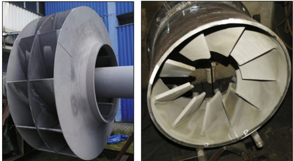
Fig. 13 Protective thermal spray coating deposited on the rotor fan and the elements of pulverized coal burner [11]
