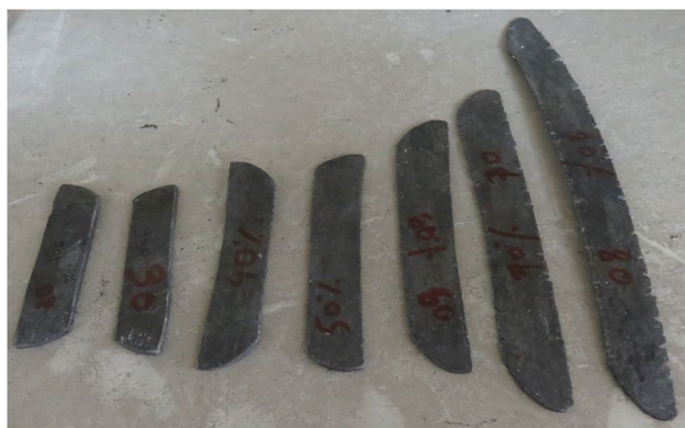
Fig. 10 Rolled plates of alloy up to 80% reduction in initial thickness
