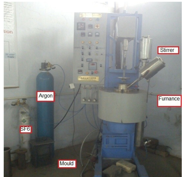
Fig. 1 Casting set-up used for fabrication of magnesium composite
