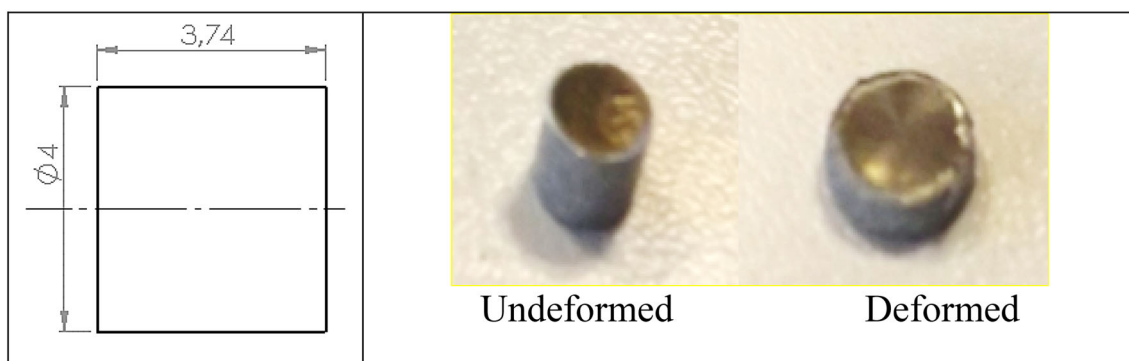
Fig. 1 Compression test sample
