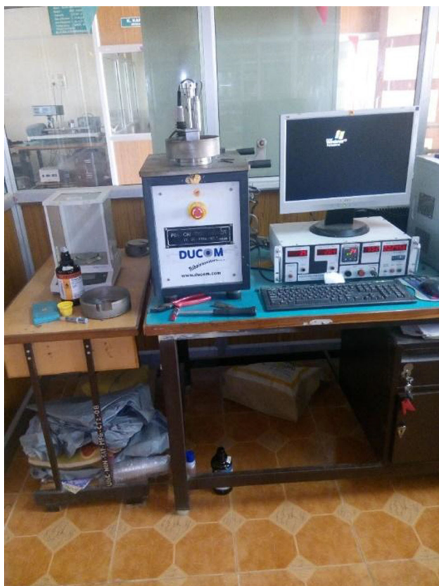
Fig. 2 Photographic image of pin-on-disc wear test machine
