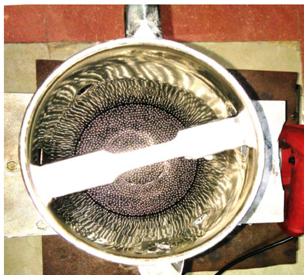
Fig. 1 Experimental set-up used for surface mechanical attrition treatment of AISI 6150 steel
