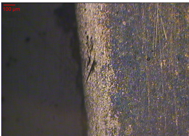
Fig. 2 Microstructure of SMATed sample reveals the thickness of severe plastic deformed region
