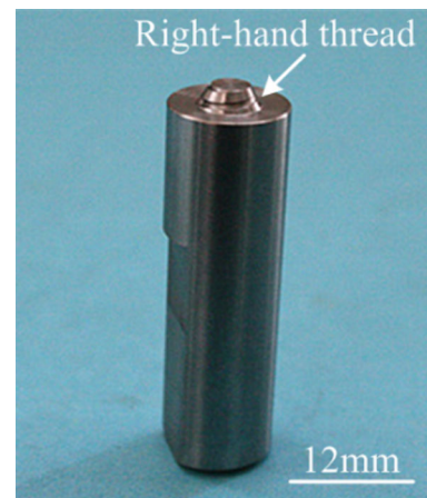
Fig. 1 Rotating tool with a threaded pin used in the present study
