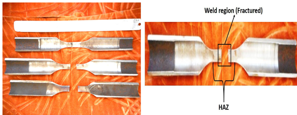
Fig. 5 Welded specimens after tensile test
