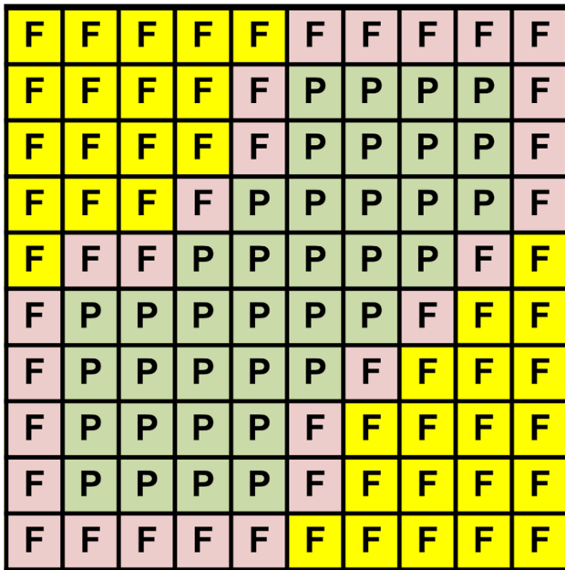
Fig. 2 Illustration of preferred nucleation sites (cells with pink shade) for austenite (F ferrite, P pearlite)
