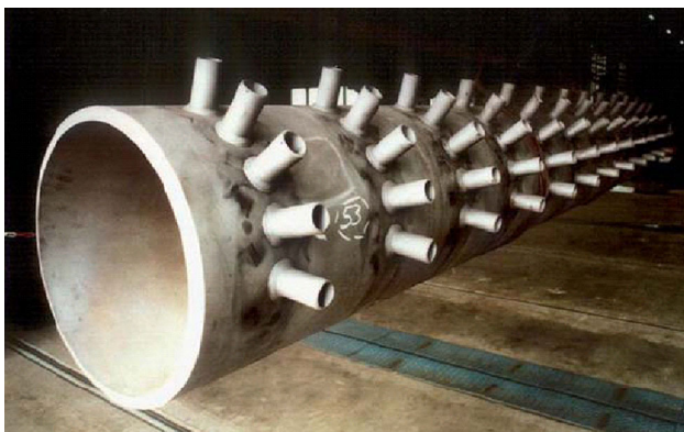
Fig. 1 Photograph of a typical high temperature boiler header [6]. Using creep strength enhanced ferritic steel reduces the thickness compared to a part made from low alloy steel
