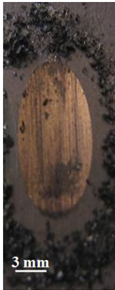
Fig. 20 Wear track of the composite C after 36,000 cycles
