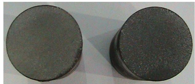
Fig. 3 Fracture surfaces of coating bond strength test
