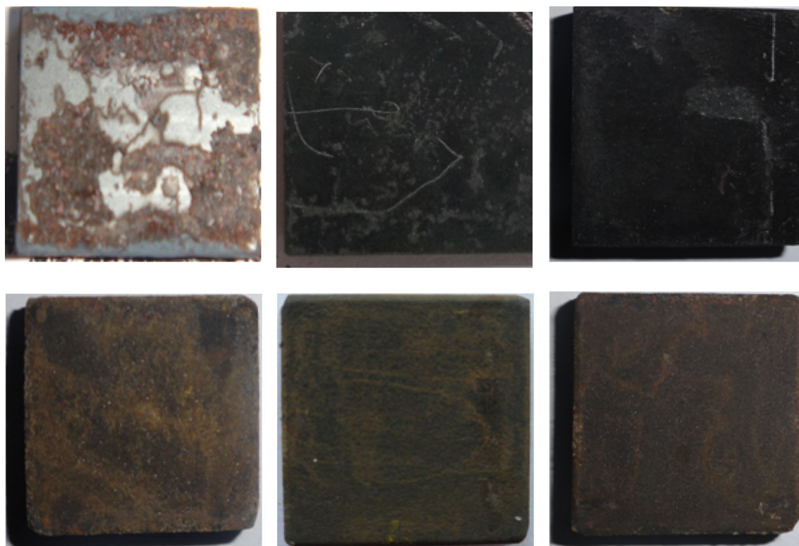
Fig. 8 Macrographs of uncoated substrates ( top row , in sequence for T22, Mdn and Superfer-800H) and (\text{Cr}_3\text{C}_2\text{-}35\% \text{ NiCr}) + 5\% \text{ Si} coating ( bottom row , in sequence for T22, Mdn and Superfer—800H) subjected to hot corrosion
