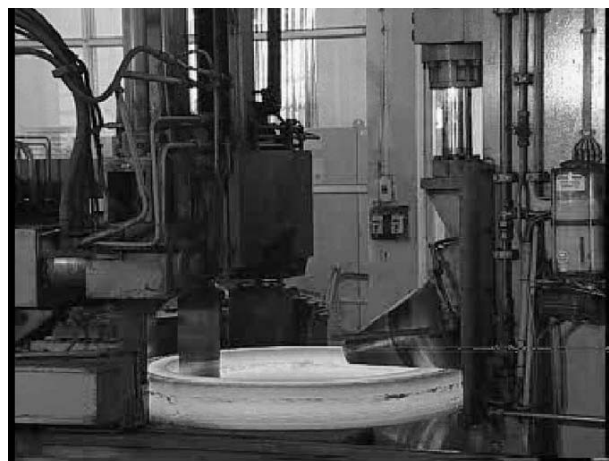
Fig. 4 : Ring rolling operation at HAL(F&F)
