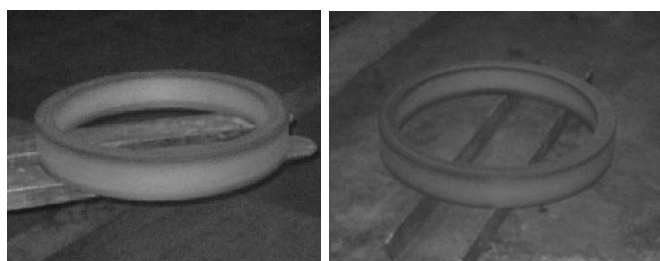
Fig. 5 : Kaveri ring forging in hot condition.
