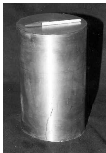
Fig. 3 : Indigenous Ti-6Al-4V forging stock [180mm diameter]
