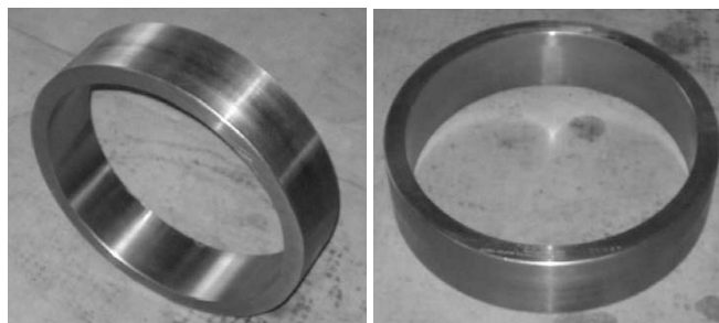
Fig. 6 : Kaveri ring forging in machined condition
