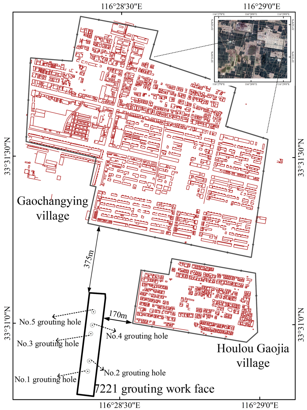
Fig. 1 Schematic of 7221 work face and grout holes parameters
