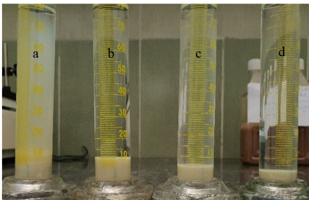
Fig. 3 Clay swelling in solutions containing a 0, b 4000, c 15,000 and d 40,000 mg/L NaCl
