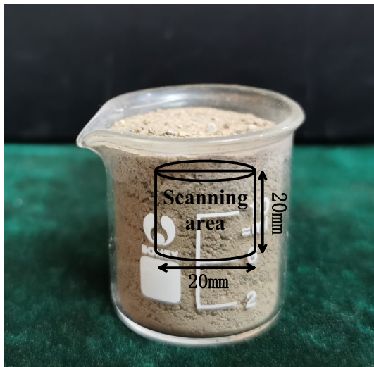
Fig. 4 Microbial consolidation of soil samples for CT scan
