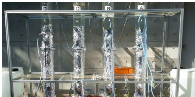
Fig. 2 Experimental set-up for column experiments showing columns wrapped in aluminum foil to prevent the effect of light
