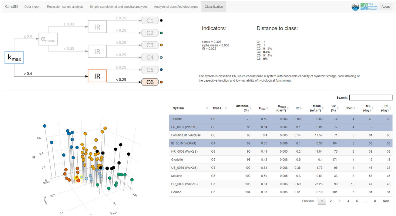
Fig. 6 Classification tab. The top part shows the classification flowchart and its associated text description: indicator values and distance to other classes (section “Classification”). The bottom part presents
