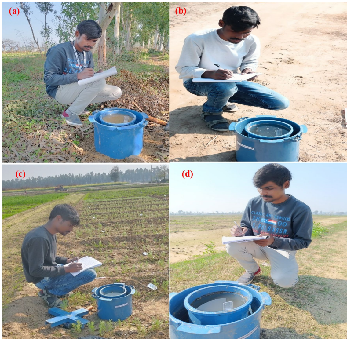
Fig. 5 Measurement of infiltration rate in the field using double-ring infiltrometer under different land-use conditions: a forest land, b hard surface land, c cultivated land and d Barren land
