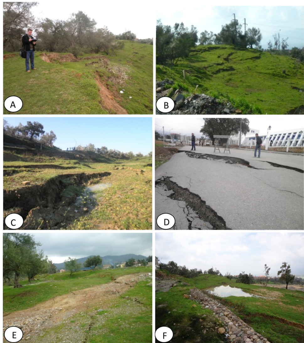
Fig. 7 Landslides deformation characteristics observed following heavy rainfall of 2012 in the vicinity of Ighil Bouzel (north of the city of Azazga): a–c scarps with an arched shape located at the medium section of the landslide body in the districts of Tala Oukouchah and Zen. d Scarps along the national road RN72 in the district of Ighil Bouzel, e tensile cracks located within the moving masses in the district of Ighil Bouzel and f collapse and stagnation of rainwater at the toe of the landslide. The locations of the photos taken ( a–h ) are shown in Fig. 9
