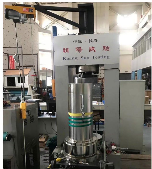
Fig. 2 GAW-2000 electro-hydraulic triaxial testing machine
