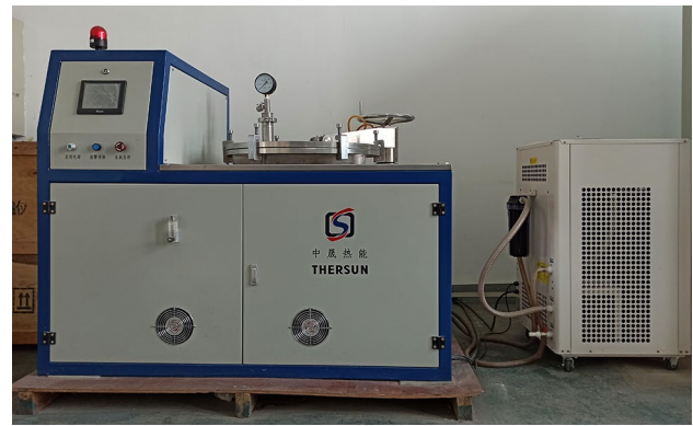
Fig. 1 RWLM6 microwave high-temperature heating furnace
