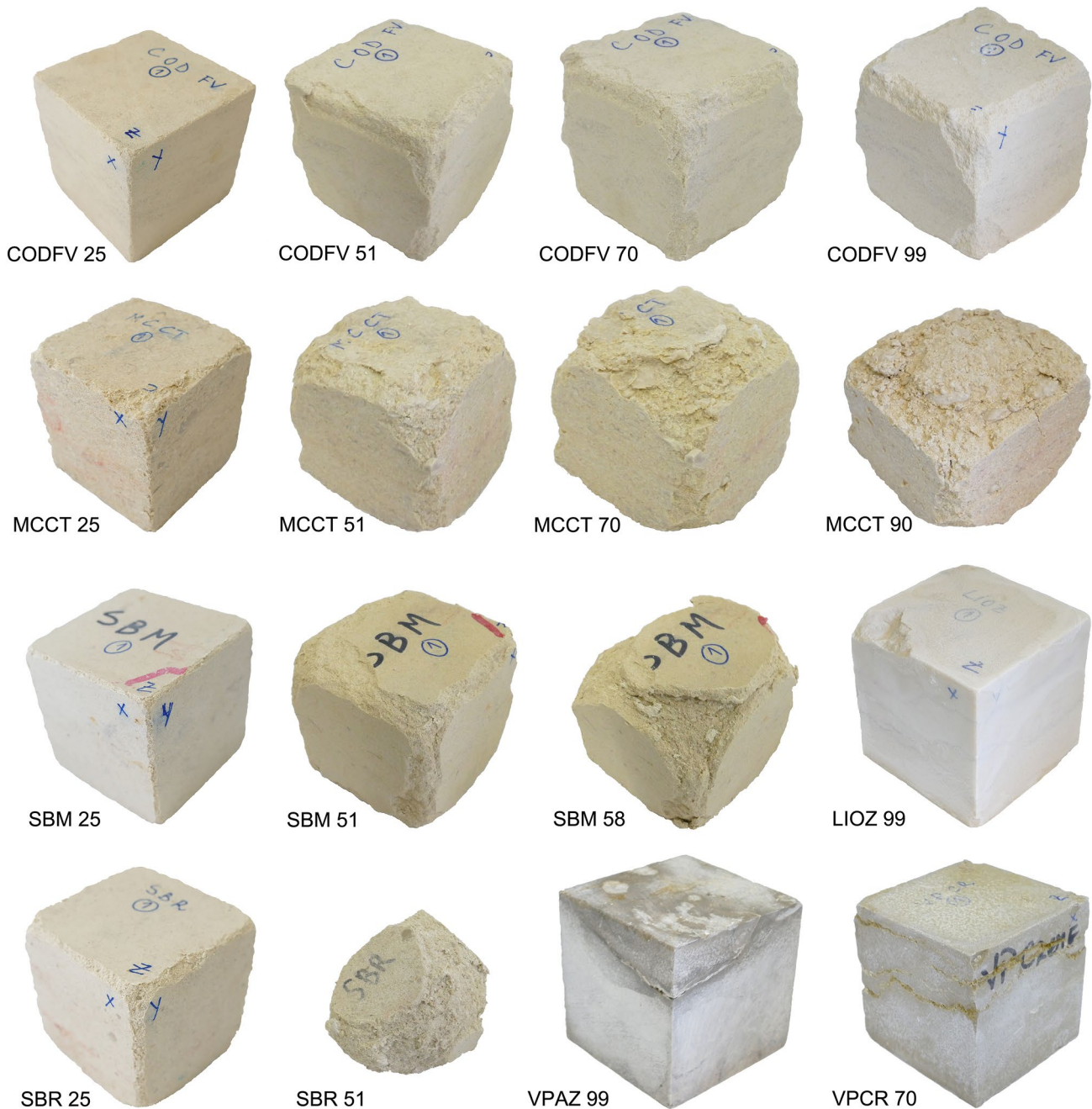
Fig. 14 Evolution of selected samples during the salt test
