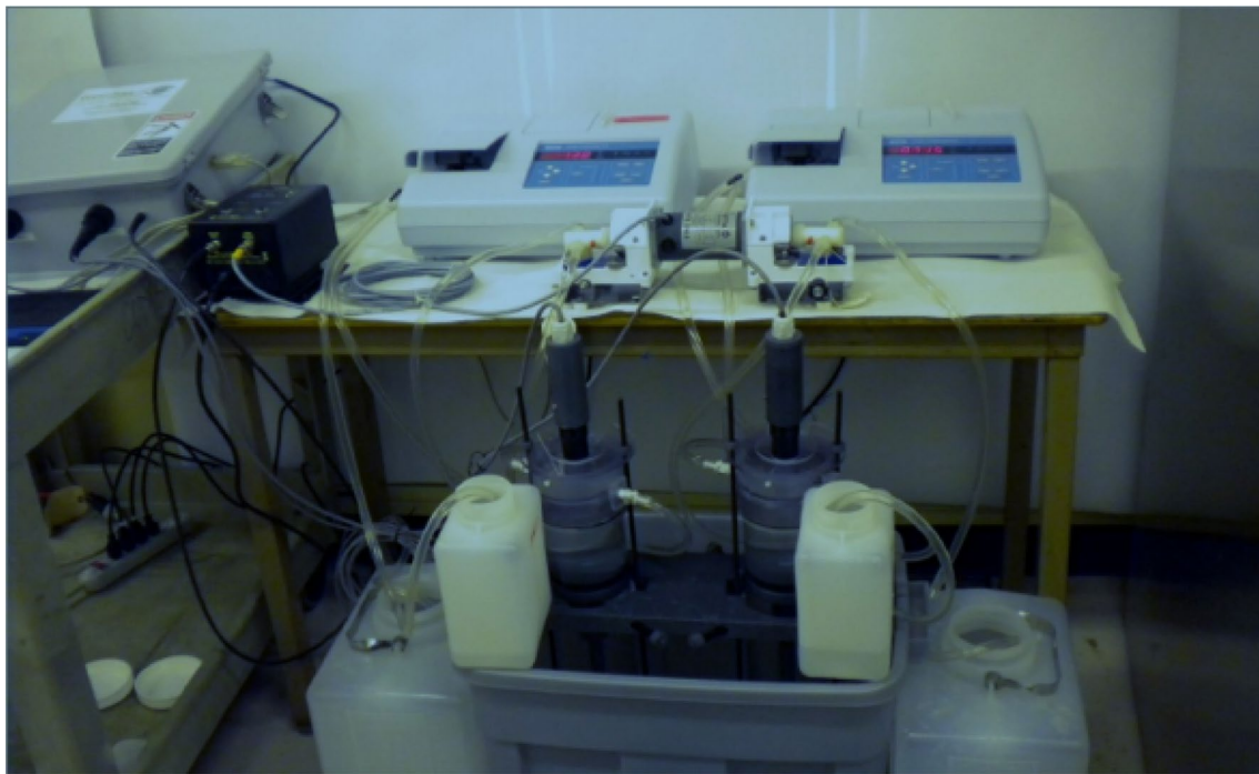
Fig. 10 Organization parameters of U-GEMS which is calculated to degree the erodibility of fine-grained sediments in a 10 cm core tube over a calibrated variety of shear pressures from 0.02–0.47 Pa (Dong et al. 2019)
