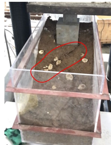
Fig. 25 Part failure of SRS
