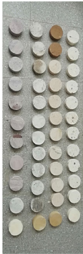
Fig. 5 An overview to disc samples before and after fracture toughness tests
