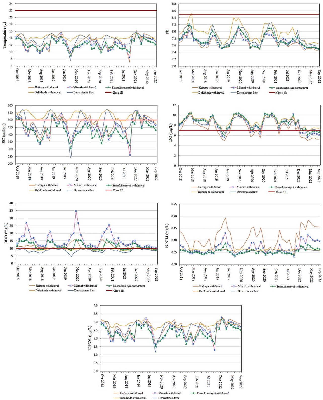
Fig. 9 The trend of quality parameters in the water withdrawal points in Dez river from 2018 to 2022 (Reference Scenario)
