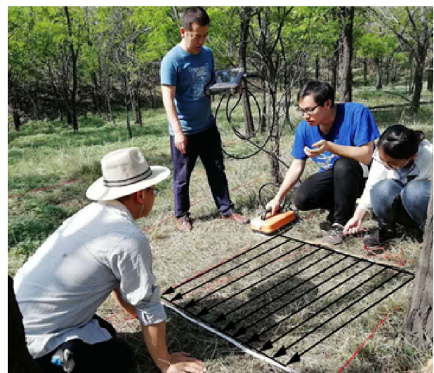
Fig. 2 Detection process with GPR
