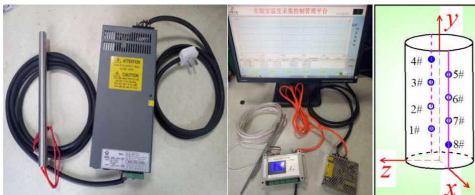
Fig. 2 The heating system and temperature measuring system diagram
