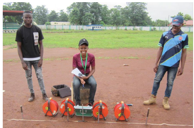
Fig. 2 Field data acquisition using Schlumberger array at the Onueke Township Stadium
