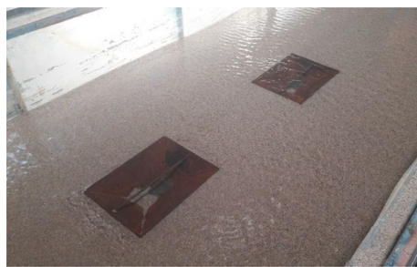
Fig. 2 Metal molds for the formation of mining pits
