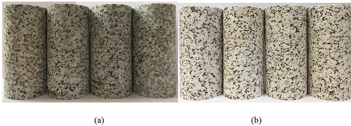
Fig. 2 Granite specimens before and after high-temperature treatment; a granite specimens before high-temperature treatment; b granite specimens after high-temperature treatment
