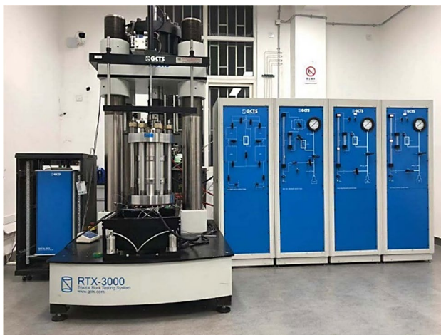
Fig. 3 RTX-3000 triaxial testing machine system for rocks
