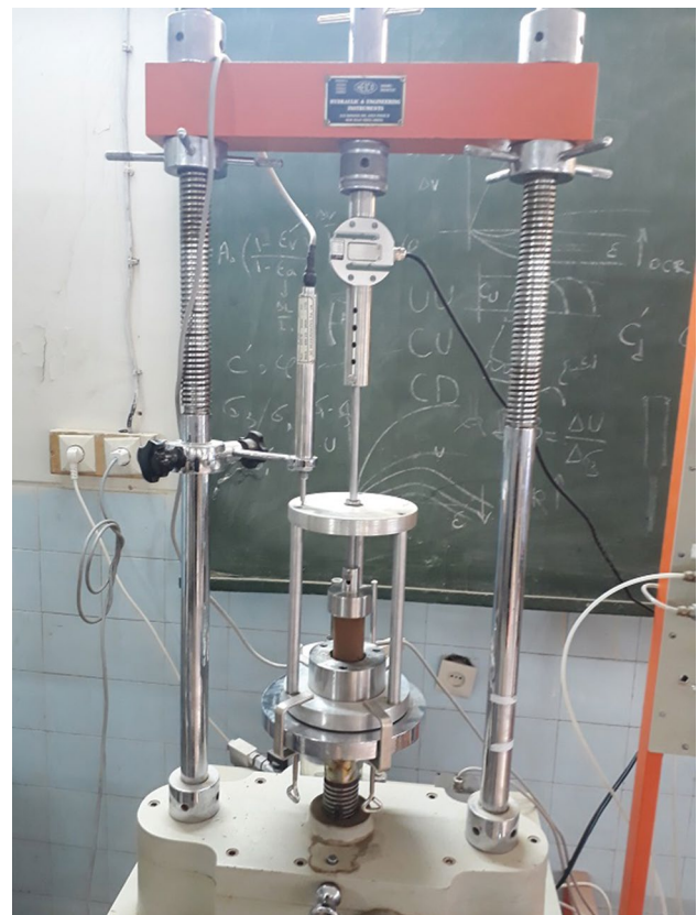
Fig. 4 Setup used for direct tensile strength test
