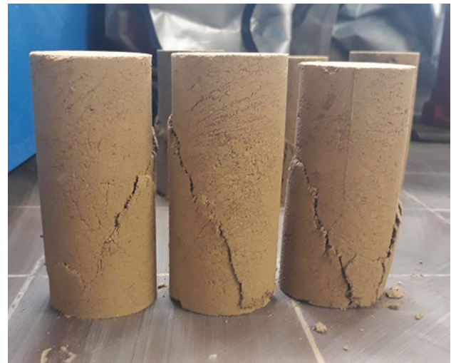
Fig. 3 Three un-treated specimens of S1 Soil after UCS test
