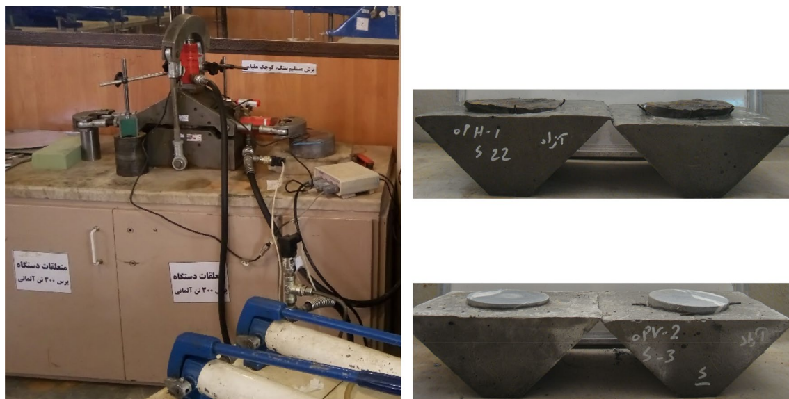
Fig. 6 a Laboratory Shear box apparatus, b rock joint sample (OPH1-S22), c saw-cut sample (OPV2-S3)
